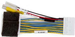
A multi-colored flat ribbon cable with a black foam pad on one end and a white connector on the other. A small white label with the ID number 873088 is visible on the cable.                                                | Кабель для подключения камеры к монитору Scion iA Connect 2016– г.в.                             |
